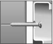
**Studs:** Secure to the wall with #12 x 2" pan head screws at stud locations.
