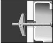
**Drywall:** Drill 1/2" holes and secure to the wall with toggle bolts.
