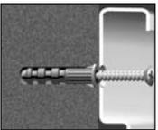
**Concrete:** Drill 1/4" holes, insert #12 wall anchors and secure to the wall with #12 x 2" pan head screws.
